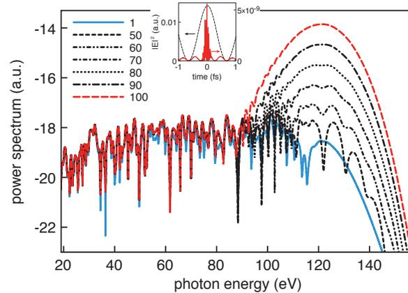
Fig. 2. XUV yield amplification obtained by filtering the harmonics spectrum at 80 eV with 120 eV spectral bandwidth. The filtered XUV is combined with the IR pulse as delayed as it comes out from the output of the interaction, in all iterations. The different lines correspond to the different iteration number, as indicated. The inset shows the filtered XUV pulse from the 100th iteration (red full line) compared with the input IR field (black dotted line).
