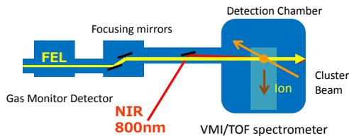
Figure 1. Schematics of experimental apparatus
