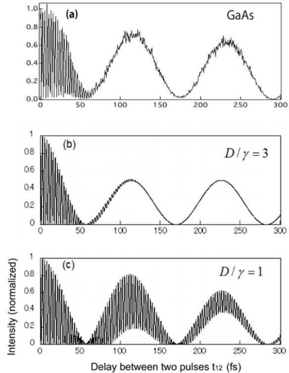
Figure 1. The interferogram for the LO phonon ; (a) experiment for GaAs at RT and (b), (c) theory.
