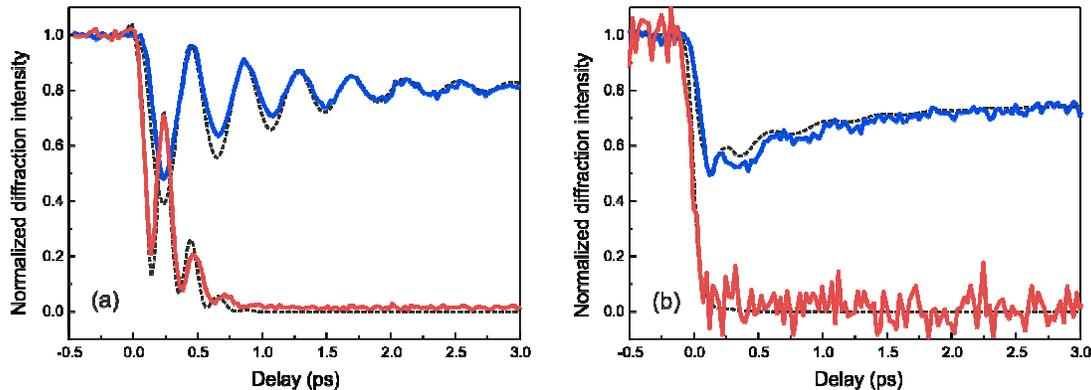
**Fig. 1.** Time dependent intensity of (a) the  $(\bar{2}\frac{1}{2}0)$  superlattice reflection measured at 6.53 keV and (b) the  $(0\bar{3}0)$  reflection measured at 6.555 keV for a pump fluence of 1.8 (blue) and 9.9 mJ/cm<sup>2</sup> (red), respectively. Dashed black lines: simulation based on a single time dependent order parameter. The simulation does not account for the significant resonant enhancement of the  $(0\bar{3}0)$  reflection due to charge order.
