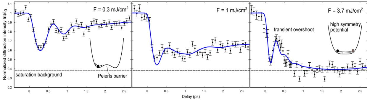
**Fig. 1.** Time evolution of (1 3.25 -0.5) SL peak diffraction intensity, normalized to the equilibrium diffraction intensity  $I_0$ . The dashed line depicts the saturation background. Errorbars correspond to photon counting statistics. Lines are fits to the model as described in the text. The low fluence data shows a clear signature of the soft mode of the system at 1.62 THz. For the highest fluence, we observe a transient overshoot.
