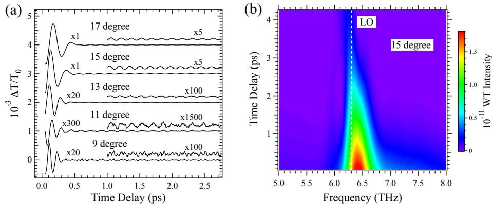
Fig. 2. (a) Time-resolved transmission changes of the CuCl microcavity obtained at various incident angles of pump pulses. (b) Image plots of wavelet transformation (WT) of the coupled oscillation extracted from time domain signals observed at the incident angle of 15 degree. The vertical dotted line indicates the LO phonon frequency of CuCl.
