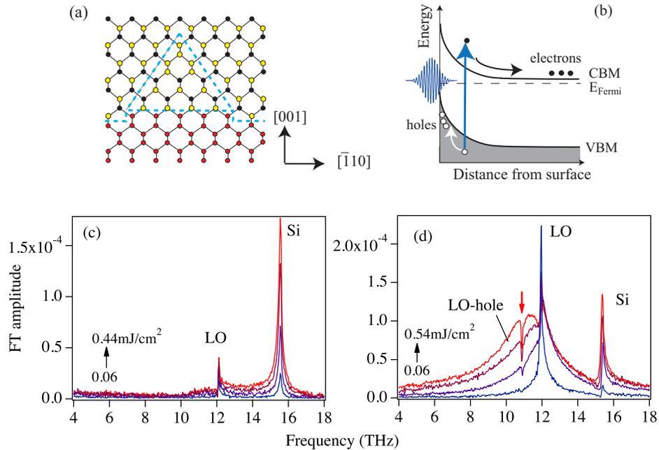
Fig. 1. (a) Atomic model for APDs on P-P exclusive  $\{111\}$  planes. (b) Schematic energy diagram of an n-doped semiconductor surface. (c,d) FT spectra of anisotropic reflectivity changes of GaP/Si(001) samples: sample II without APD (c) and sample I with APDs (d).
